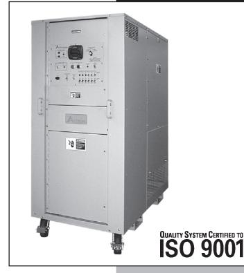
he Avtron Patriot Load Bank is a portable, self-contained unit that simulates electrical loads. It is ideal for routine load testing of standby diesel generating systems at remote sites or for factory production line testing of (UPS) Uninterruptible Power Supplies, turbines, or engine generator sets. This model provides resistive loading up to 700 KW at either 240/480 Volts AC in a convenient, and easy-to-use package.
