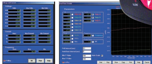
Avtron ADMS Digital Meter, Real-Time Data Logging and Trending Screens.
