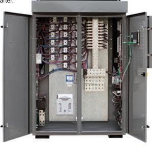
The load bank enclosure is of double wall construction for cool exterior and thermal isolation of the load elements. Cooling airflow through the enclosure is vertical with cold air intake at the bottom and hot air exhaust out the top. Intake and exhaust openings are screened. Enclosure is powder-coated dark gray. Hood powder-coated high temperature black
