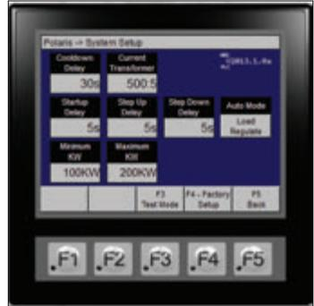
**Figure 31 System Setup Screen**
