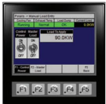
Figure 27 Manual Load Entry Screen
