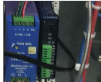
Figure 10 Serial Adapter
