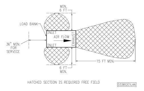
Figure 3-1. Load Bank Installation Airflow Clearance Requirements
