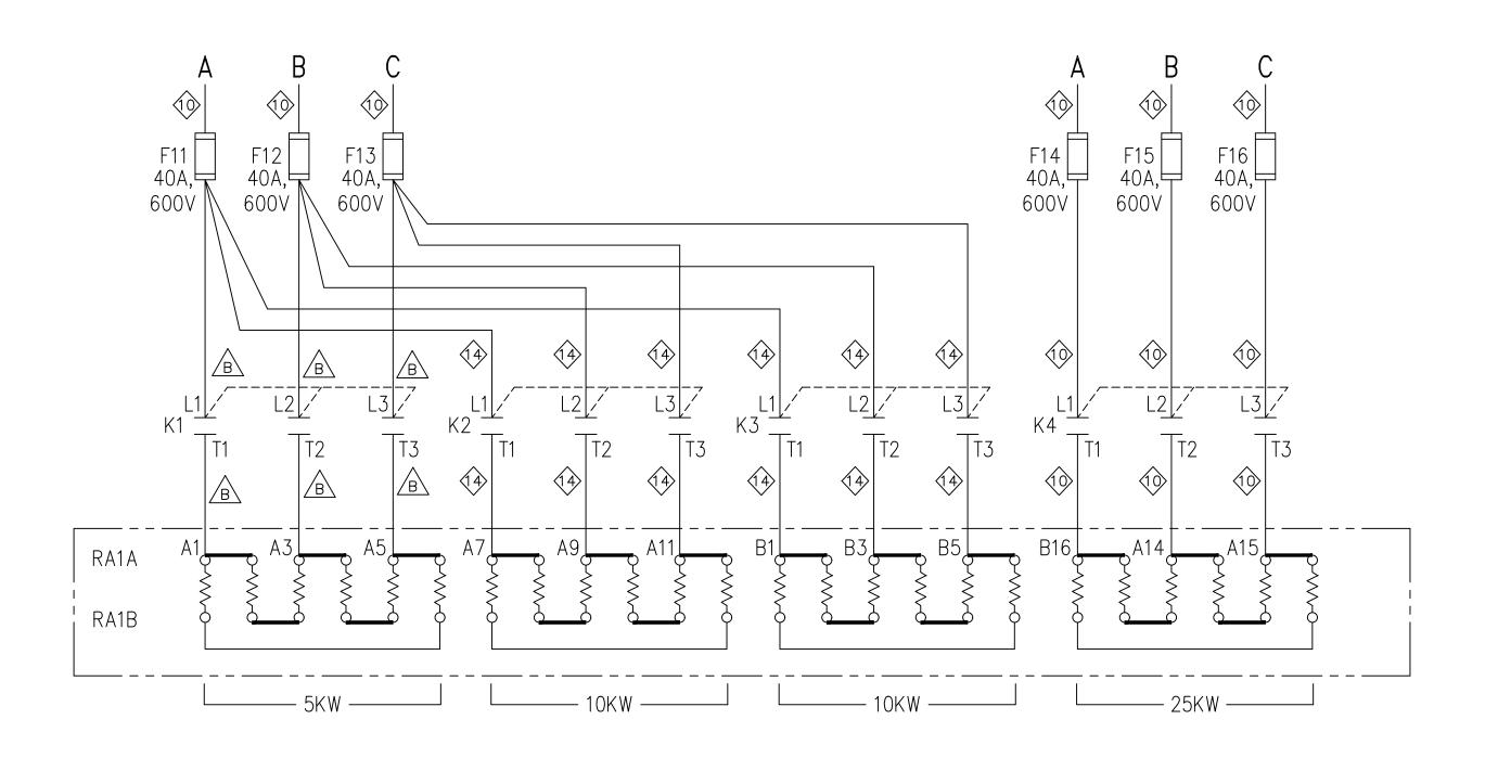
NOTE: WIRES FROM BUS BARS A,B, & C TO FUSES ARE ALL INDIVIDUAL RUNS. BOLD LINES FROM FUSES INDICATE DIRECT CONNECTION TO RESPECTIVE BUS BARS.
