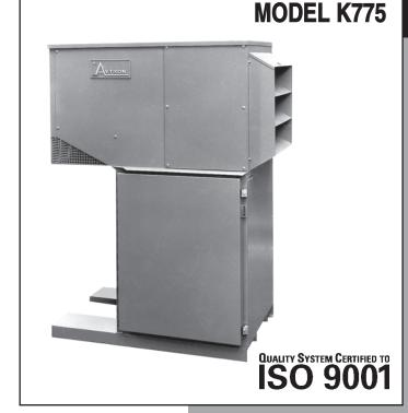
he Avtron Model K775 load bank is designed for permanent outdoor installation, providing 15 KW to 75 KW of load at 240 or 480 volts, 3-phase. Its four wire wye configuration allows for simplified single-phase testing applications. The K775 series is built using the latest, state-of-the-art load bank technologies to provide years of reliable operation.
