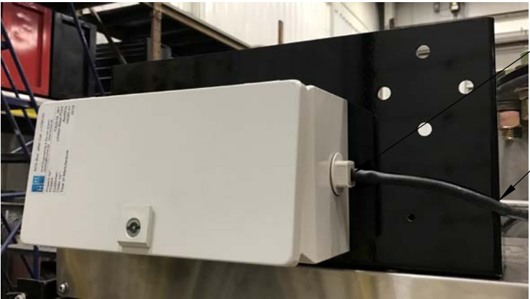
GP1815-18 - PRESSURE TRANSMITTER BRACKET - SHIPPED BOLTED TO SCR
