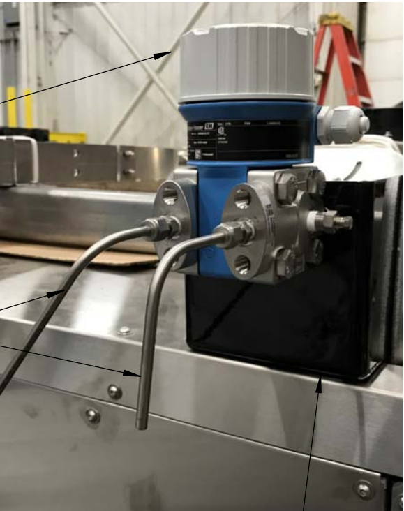
GP1815-18 - PRESSURE TRANSMITTER BRACKET - SHIPPED BOLTED TO SCR
